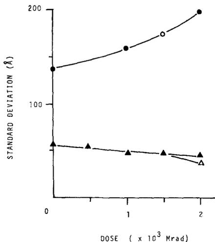
Figure 8 Standard deviation of the crystallite size distribution function. Circles: 110, triangles: 002. Open circles and triangles are for irradiation in vacuum.
