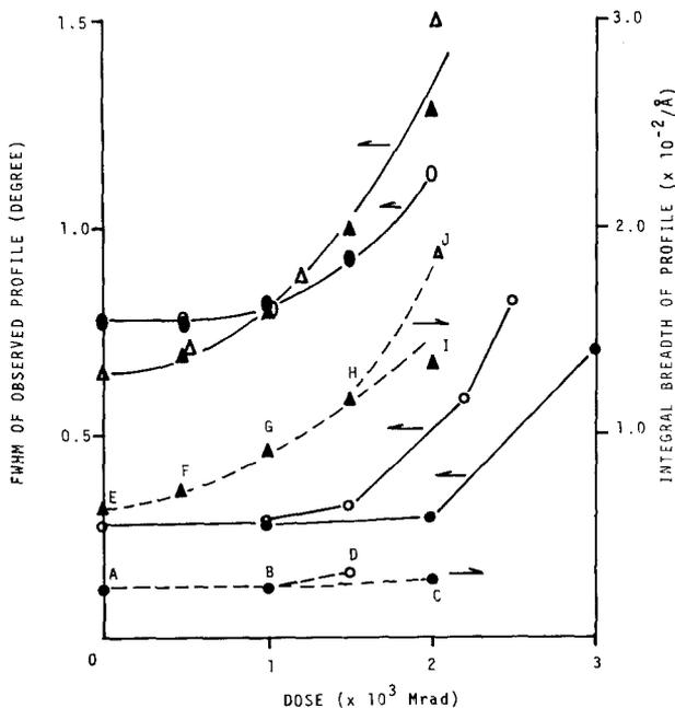
Figure 2 FWHM (solid lines) and integral breadth (dashed lines) of profile. ●: 110 of unoriented LPE, irradiated in air, ○: 110 of unoriented LPE, irradiated in vacuum. 0 and 0': 110 of oriented LPE, irradiated in air and in vacuum, respectively. ▲ and △: 002 of oriented sample, irradiated in air and in vacuum, respectively.
