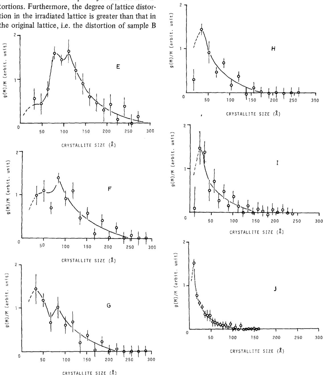
Figure 5 Crystallite size distributions in the chain direction. E: unirradiated sample, F: 488 Mrad irradiated sample, G: 1017 Mrad irradiated sample, I: 2000 Mrad irradiated sample, J: 2020 Mrad irradiated (in vacuum) sample.
