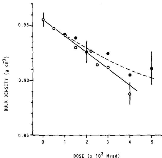
Figure 10 Changes in the bulk density of the sample. Closed circles: irradiated in air; open circles: irradiated in vacuum.
