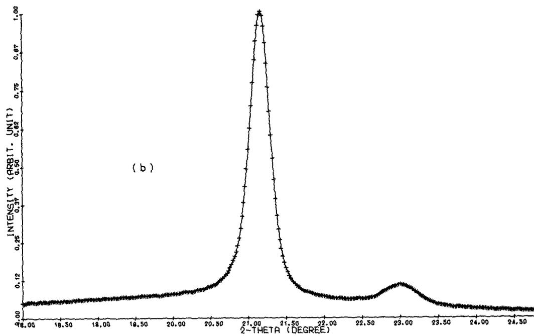
Figure 1 Examples of irradiated profiles. (a) Unoriented 110 profile, (b) 110 profile of 2000 Mrad irradiated sample, (c) unirradiated 002 profile, (d) 002 profile of 2000 Mrad irradiated sample.
