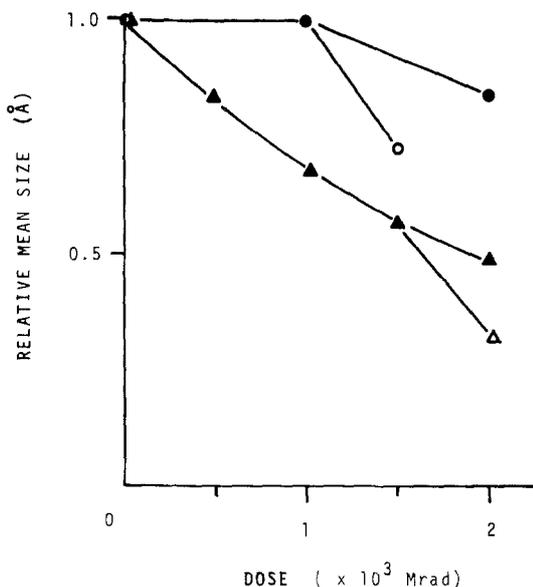
Figure 7 Changes in the mean size. ● and ○: relative mean sizes in the lateral direction, irradiated in air and in vacuum, respectively. ▲ and △: relative mean sizes in the chain direction, irradiated in air and in vacuum, respectively.
